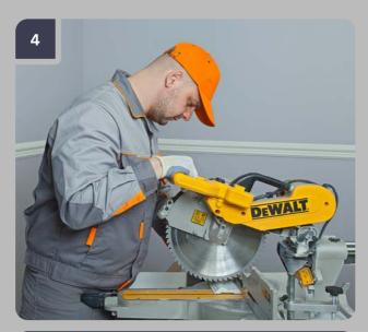
Set the angle on the trimming saw, make a cut on the product. In rooms with 90° corners it is possible to use a mitre box and a hand saw.
